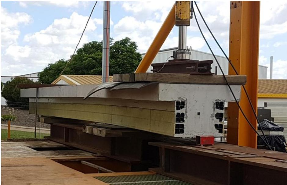
**Fig. 13** Test 3: Actual cantilever testing being undertaken on full scale prototype
