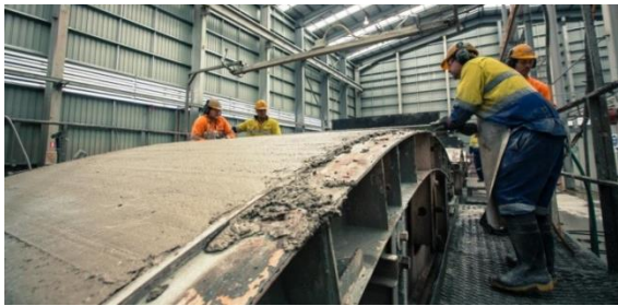
EFC segments produced in a carousel factory, Brisbane Australia
