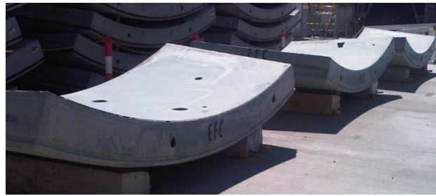
EFC segments produced in a carousel factory, Brisbane Australia
