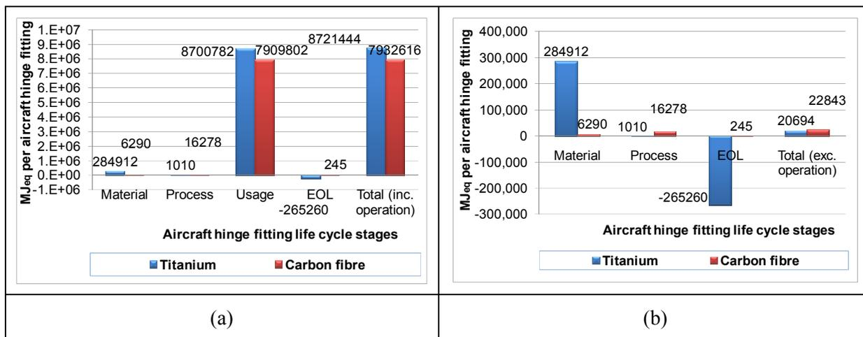
Figure 8.11: Embodied energy of the two aircraft hinge fittings in a unit of MJ<sub>eq</sub>.
