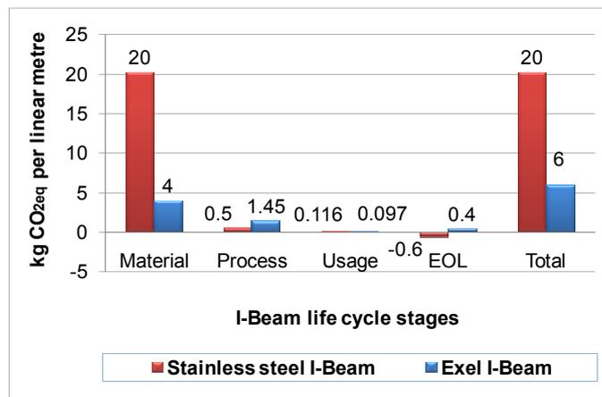
**Figure 6.12:** Comparison of the embodied energy of an I-Beam made from two different materials measuring 1 linear metre using the IPCC GWP 100a method
