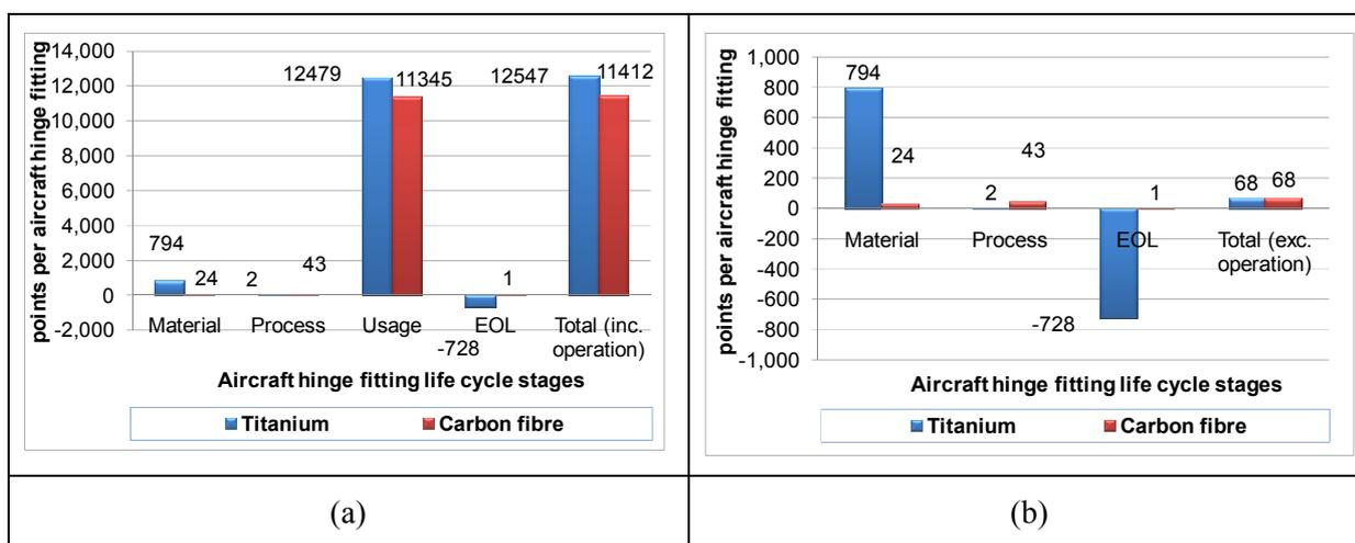
Figure 8.13: Embodied energy results of the two aircraft hinge fittings in a unit of points.
