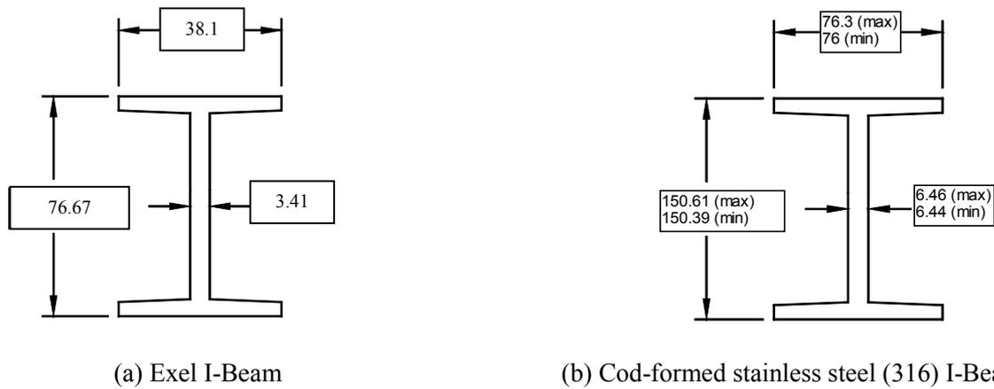
**Figure 6.6:** The dimensions of the two different I-Beams (*All dimensions are in millimetres*)
