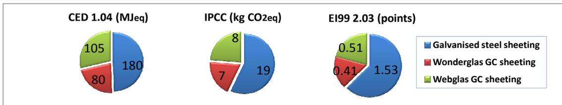
**Figure E.6:** Comparison of 1 square metre of roof sheet manufactured from glass reinforced plastic, namely Wonderglas GC and Webglas GC from Ampelite Fibreglass Pty Ltd as well as galvanised steel sheeting.
