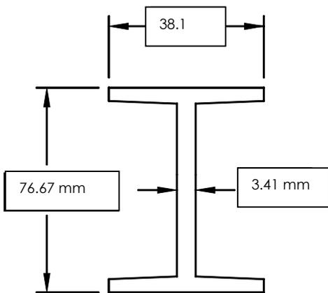
Cross-sectional area of I-beam = 498.03 mm<sup>2</sup>
