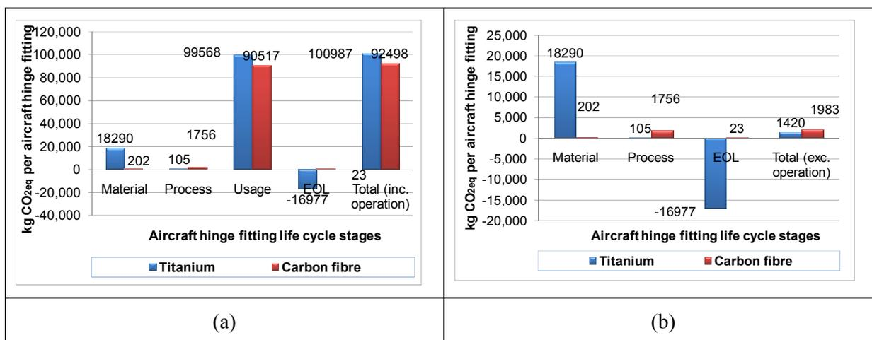
Figure 8.12 Embodied energy results of the two aircraft hinge fittings in a unit of kg CO<sub>2eq</sub>.
