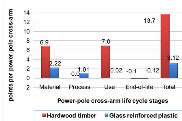
**Figure 7.10:** Comparison of the embodied energy results of the power-pole cross-arm in a unit of points.
