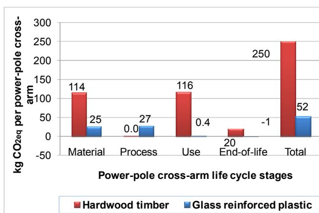
**Figure 7.9:** Comparison of the embodied energy results of the power-pole cross-arm in a unit of kg CO<sub>2eq</sub>.
