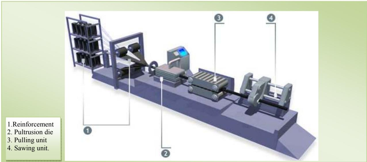
Figure 6.2: Pultrusion process<sup>44</sup>
