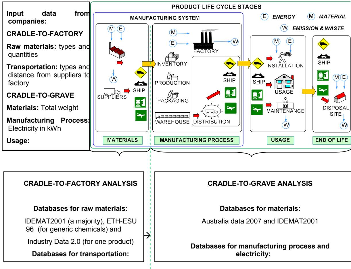
Figure 2.6: Detailed input data required for Life Cycle Assessment.
