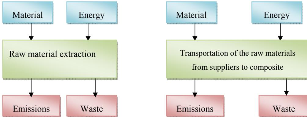
**Figure 1.1:** Input-output model of the cradle-to-factory analysis
