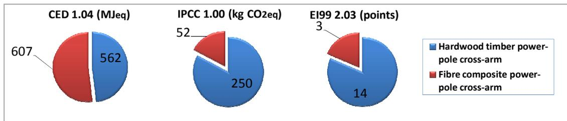
**Figure E.9:** Comparison of a 2.5 linear metre power-pole cross-arm manufactured from glass reinforced plastic of Wagners CTF Manufacturing Pty Ltd and hardwood timber.
