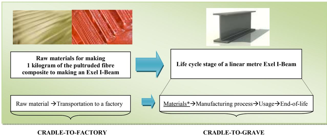
**Figure 6.3:** Scopes of cradle-to-factory and the cradle-to-grave analyses.
