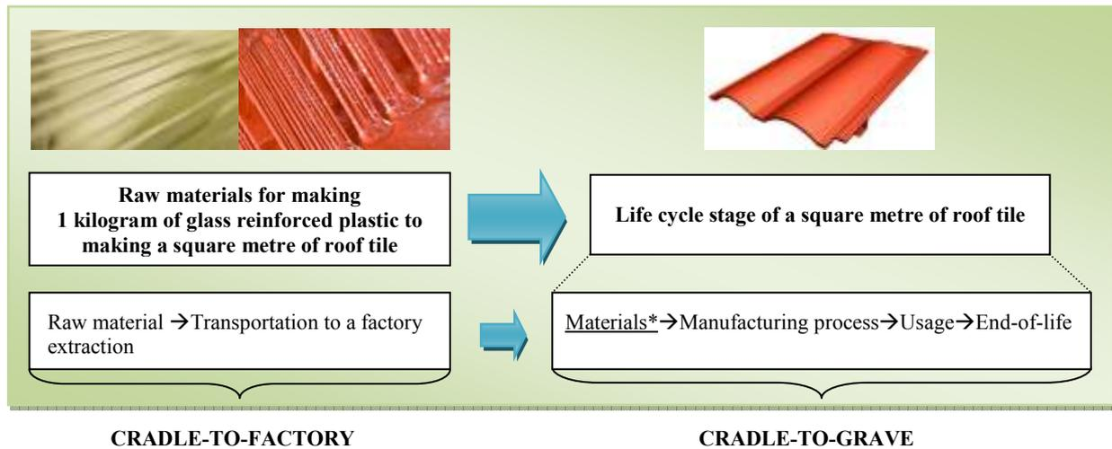
Figure 3.3: Scopes of the cradle-to-factory and the cradle-to-grave analyses<sup>7</sup>.
