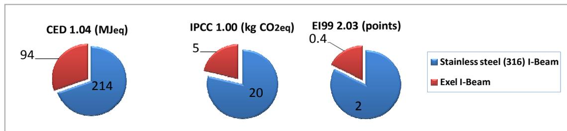
**Figure E.8:** Comparison of a 1 linear metre I-Beam manufactured from glass reinforced plastic of Exel composites and stainless steel (316).
