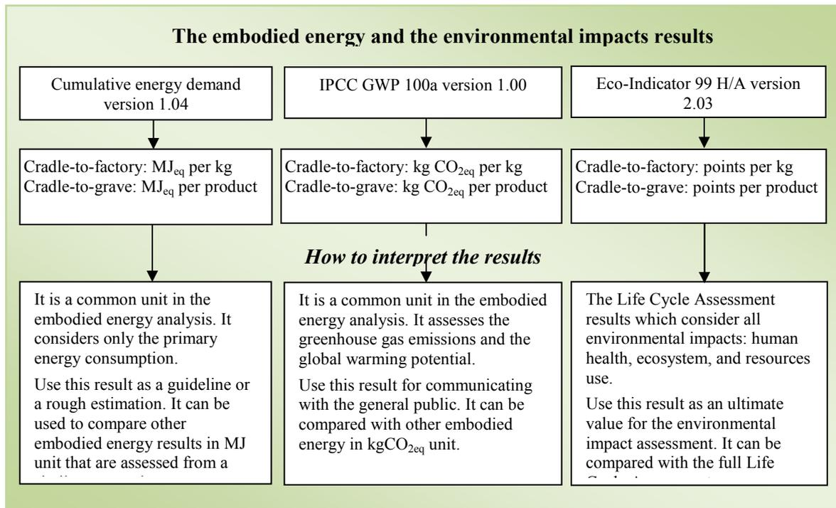
**Figure 1.3:** Diagram of How to interpret the embodied energy results
