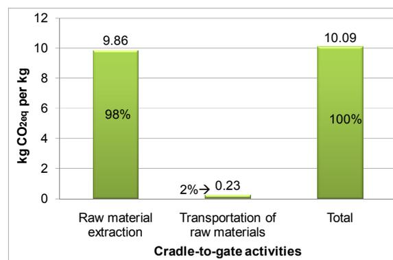
(b) Greenhouse gas emission results in kg CO<sub>2eq</sub> per kg
