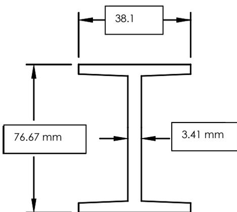
Cross-sectional area of I-beam = 498.03 mm<sup>2</sup>
