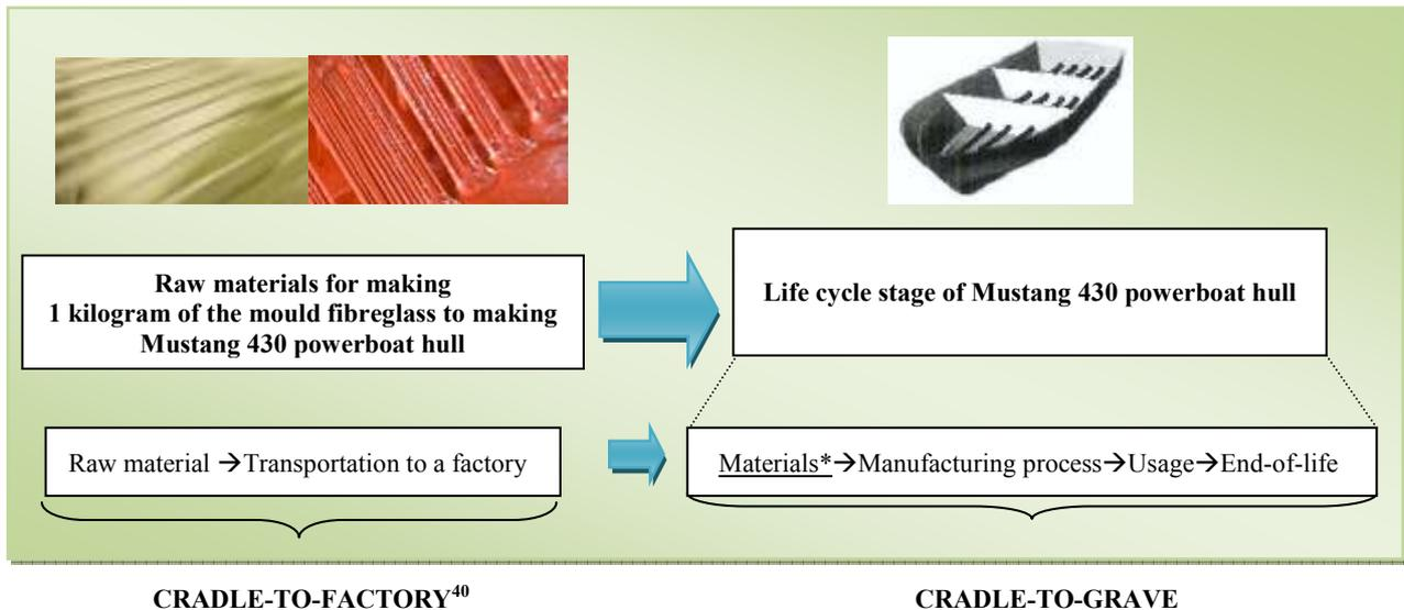
Figure 5.3: Scopes of the cradle-to-factory and the cradle-to-grave analyses.
