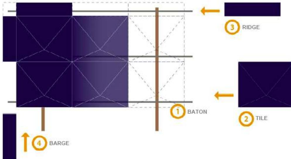
**Figure 3.2:** Installation system of the Tractile roof tile
