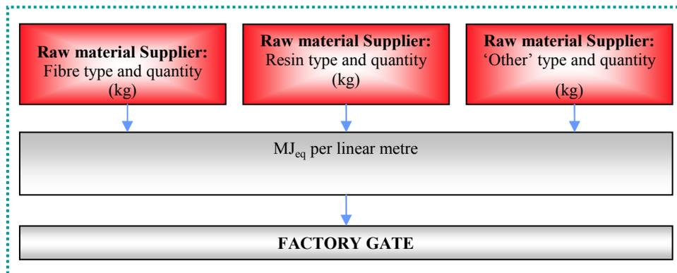
**Figure 2.7:** Block diagram of the cradle-to-factory analysis
