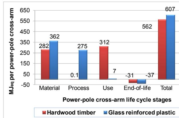
**Figure 7.8:** Comparison of embodied energy results for the power-pole cross-arms in a unit of MJ<sub>eq</sub>.
