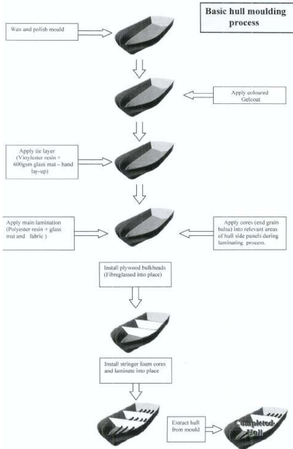
Figure 5.2: A basic hull moulding process.<sup>38</sup>
