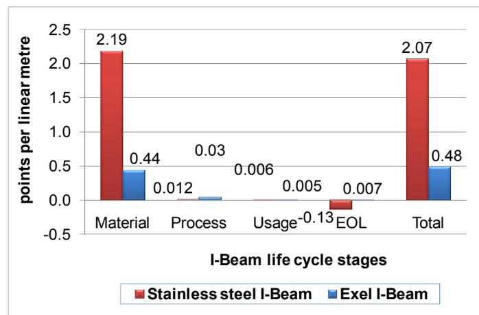
**Figure 6.13:** Comparison of the embodied energy of an I-Beam made from two different materials measuring 1 linear metre using the Eco-Indicator99 H/A version 2.03 method
