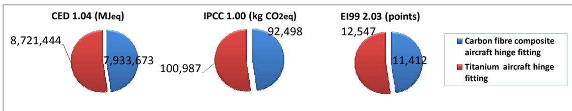
**Figure E.10:** Comparison of an aircraft hinge fitting manufactured from carbon fibre reinforced plastic of Boeing Research and Technology and titanium.
